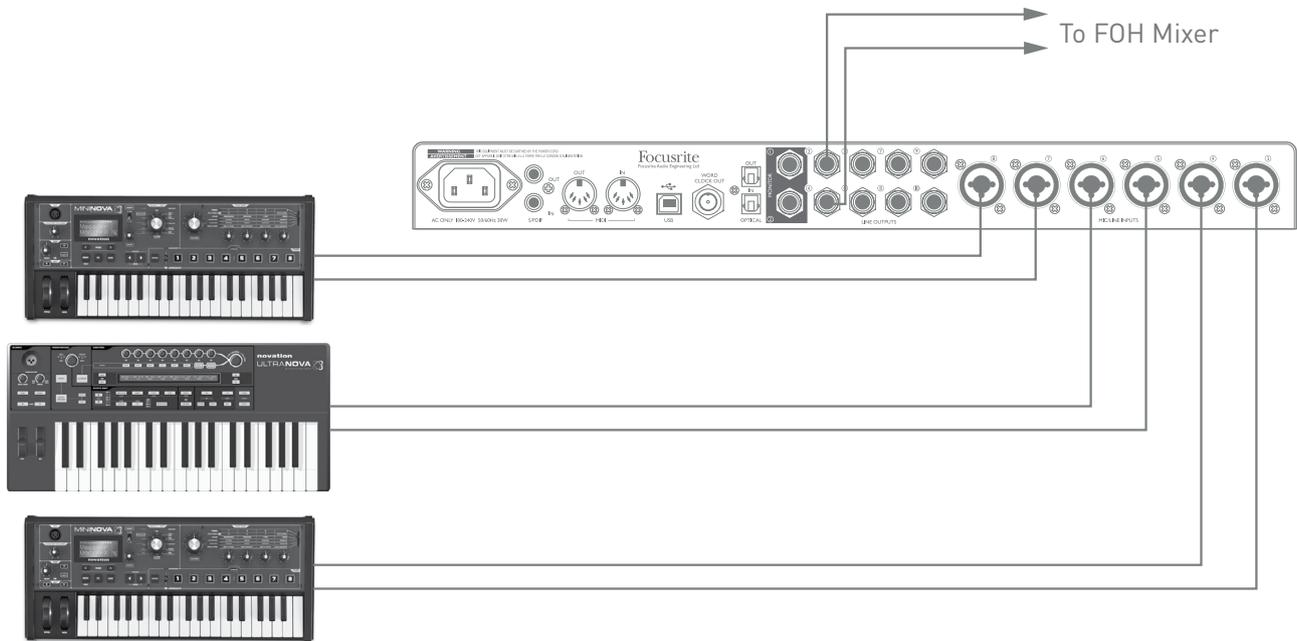
In the example illustrated, three stereo keyboards are connected to the rear panel inputs of the Scarlett 18i20; Outputs 3 and 4 go to the main PA system. The performer can adjust the volume of the individual keyboards from the front panel; he/she can also adjust the overall level of the keyboard mix.
