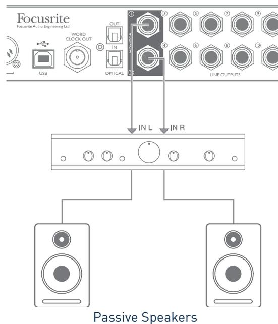
All the line output connectors are 3-pole (TRS) 1/4" (6.35 mm) jack sockets, and are electronically balanced. Typical consumer (hi-fi) amplifiers will probably have unbalanced inputs, either on phono (RCA) sockets, or via a 3.5 mm 3-pole jack plug intended for direct connection to a computer. In either case, use a suitable connecting cable with jack plugs at one end.
